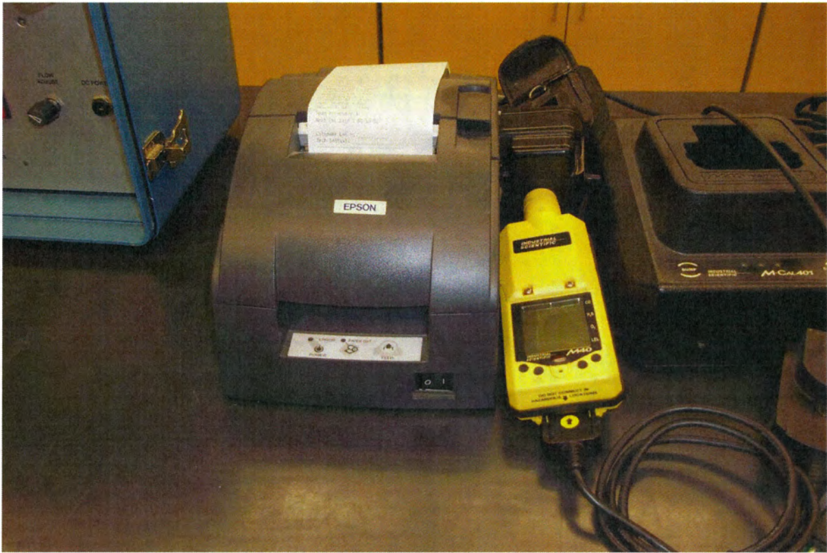
Gas Air Monitor & Calibration Station (4)
